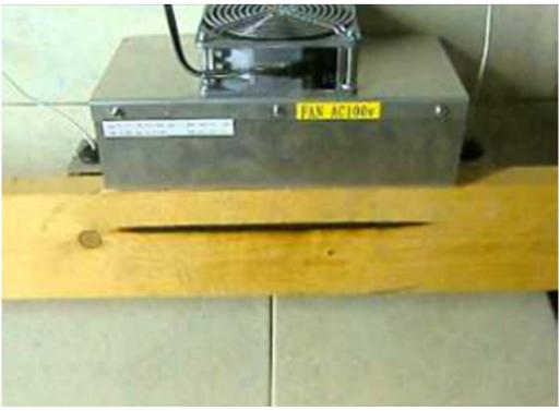
Can be varied to AC0v - AC220v in large volume of manual variable power supply. Variable of the electric power is carried out by voltage adjustment, and heating temperature can be adjusted.
